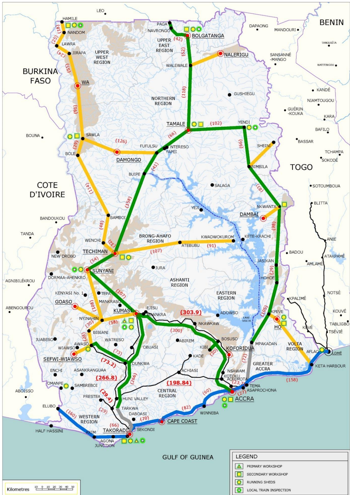
Figure 3-15. Locations for Maintenance of Railway Network
