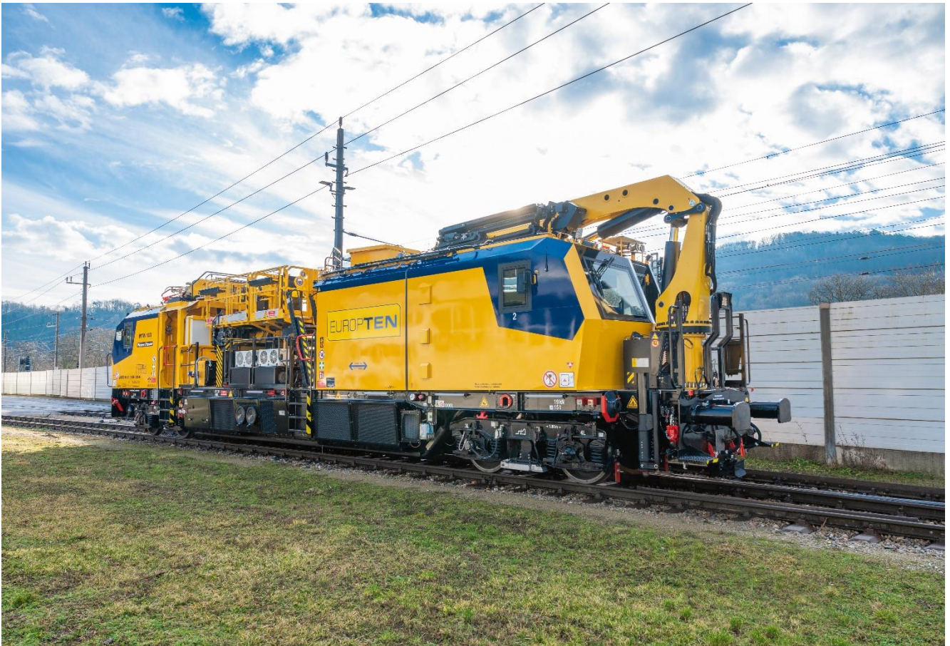
The motorized power wagon with PALFINGER equipment in action. © Plasser & Theurer
